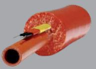
The ideal for maintaining sanitary hot water in the pipeseliminating the recirculation pumps and related equipment in centralized. It's a cable semi-conductive matrix that can be cut to length and spliced derivative, does not produce dangerous overheating even if superimposed produces a power that decreases with increasing ambient temperature.
